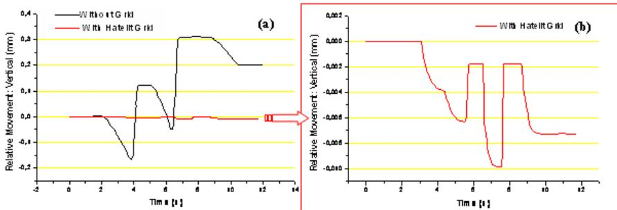
Figure 5. Vertical relative displacements between crack walls: (a) cracks on areas with and without geogrid, (b) zoom of the results on the area with geogrid.
