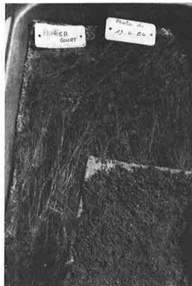
Photo 4 : On 13.4.84. A corner of seeded layer is folded up. Notice the important lot of sand trapped by the roots.
