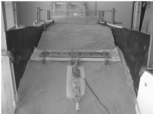
Figure 5. Photo of the implementation of an anchoring test
