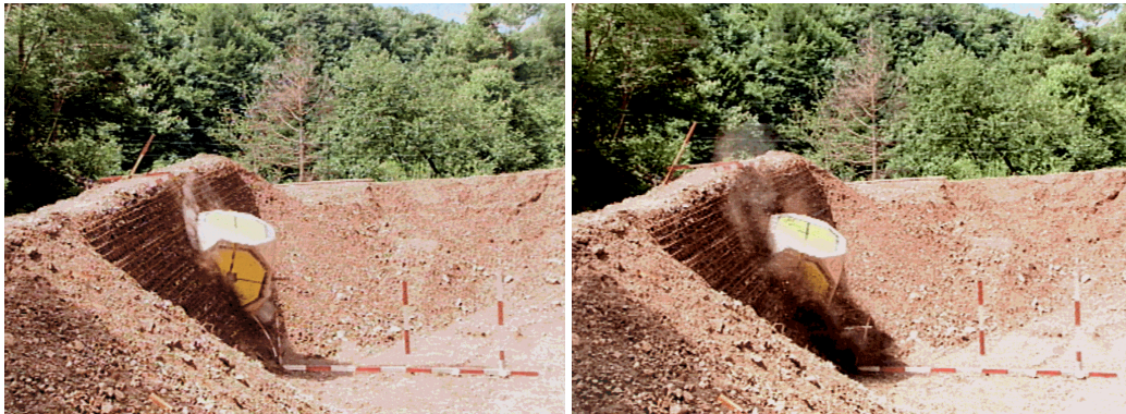
Fig. 7: Two frames showing the 8778 kg block while being arrested by the wall during the second test.
