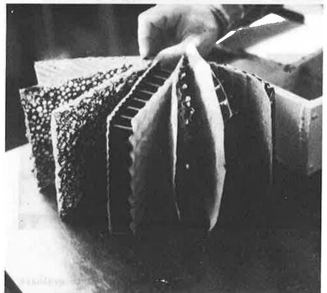
Fig. 1. - Various types of prefabricated drainage composites (or drainage geocomposites)
