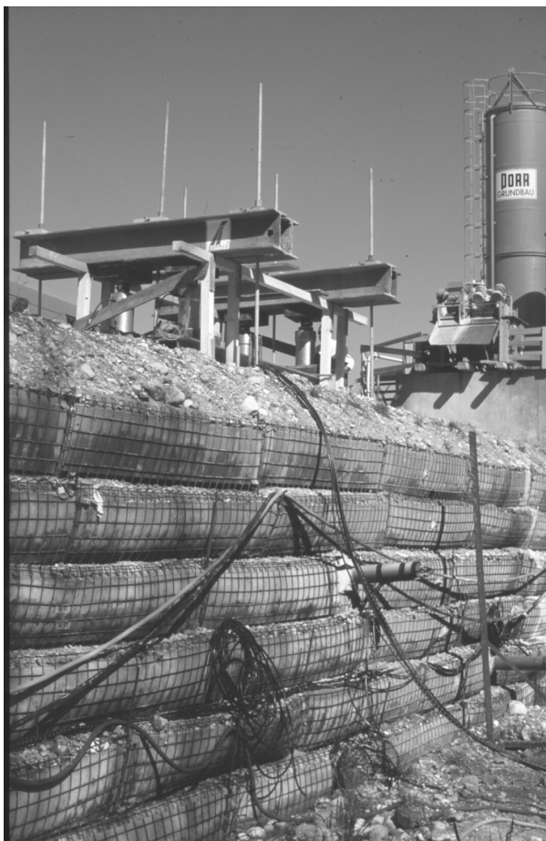
Figure 7: Cross section with loading system
