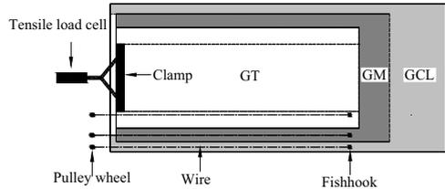
Fig. 2 Tension and displacement measure systems
