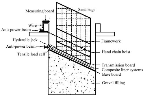
Fig. 1 The large-scale ramp test apparatus
