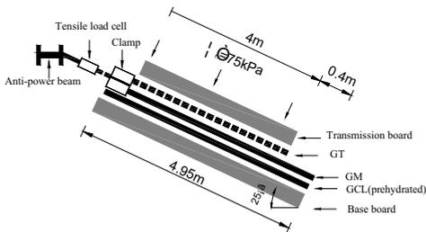
Fig. 3 GT/GM/GCL liner system test
