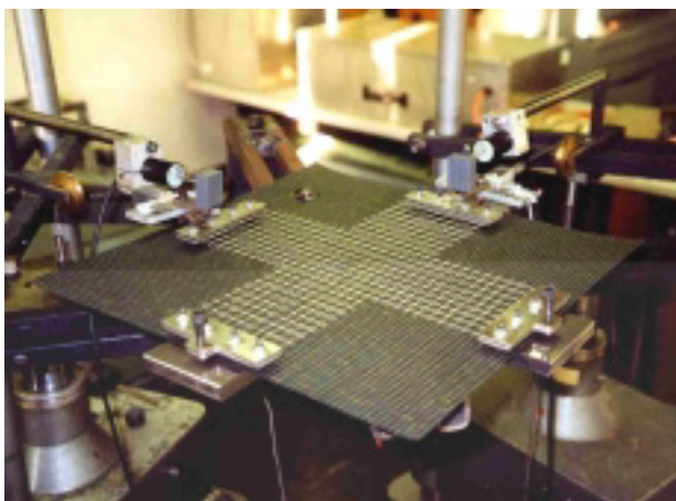
Plate 1 Biaxial test apparatus with clamped specimen
