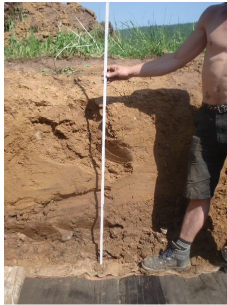
Figure 2. Cover soil in landfill B
