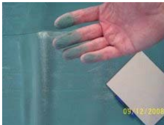
Figure 4. Chalking on surface (Courtesy DSWA)
