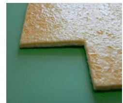
fig. 3: Swelling nonwoven with polymer powder
