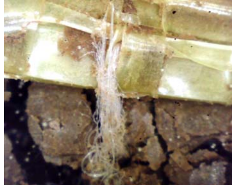
Figure 6. Enlarged view of GCL A after hydration: Failed filament
