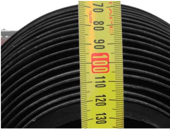
Figure 2. Embossed geomembrane roll in profile showing space created by spikes
