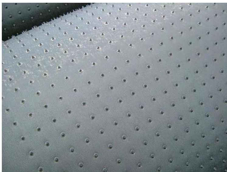
Figure 1. Embossed geomembrane (AGRU Structure Spike)
