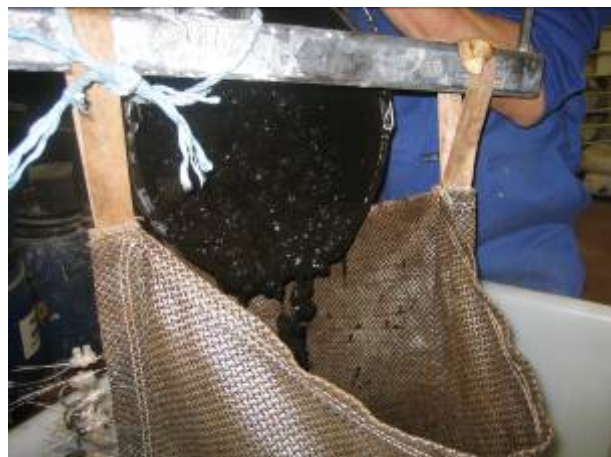
Figure 2a. Water clarification sludge – gelatinous in nature
