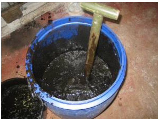
Figure 2a. Water clarification sludge – gelatinous in nature
