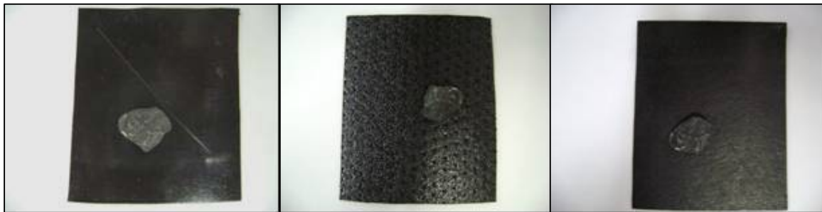
a) Smooth Geomembrane b) High-asperity textured GM c) Low-asperity sand impregnated GM
