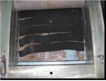
Figure 5. Geosynthetic fix system suggested by standard ISO 12957-1: 2005. Bottom steel support 300x300 mm
