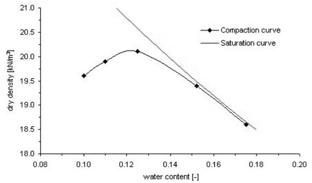
Figure 3 Compaction curve for soil mix A
