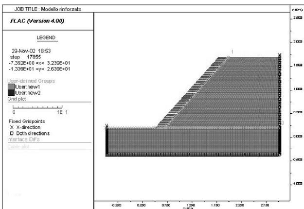
Figure 14 Considered mesh for reinforced steep slope
