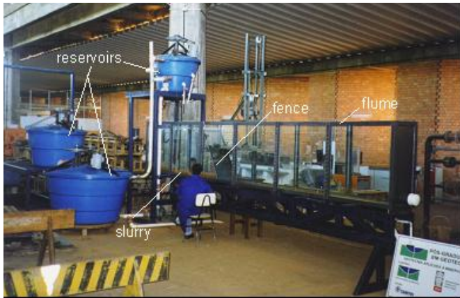
(b) Large flume during one of the tests performed
