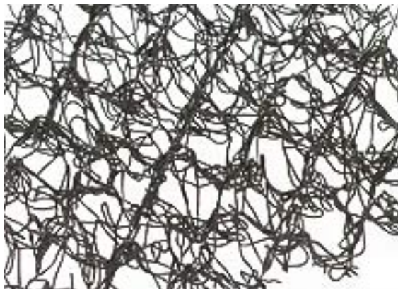
Figure 1. Structure of the tested erosion mattresses
