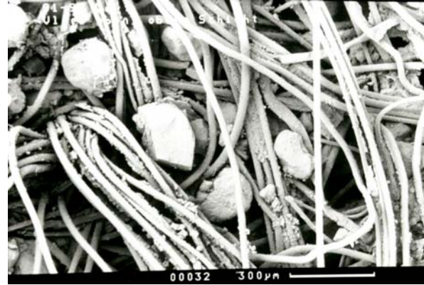
Figure 2. REM of nonwoven for excavated GDS from landfill BU (left) and landfill VI (right)
