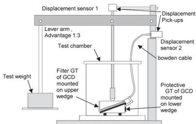
Figure 2. Schematic drawing of a test stand for determining long-term shear strength.
