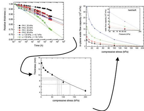
Figure 1. Illustration of the selected procedure for assessing the long-term water flow capacity under differing bedding conditions. One observes: the extrapolation of the creep curve is only then permissible when it can be shown that aging over the period being extrapolated does not invoke any relevant changes in the material due to aging.
