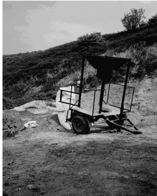
Photograph 2 Bag Filling Frame
