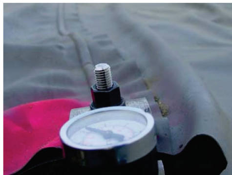
Figure 5. Inflated PVC air channel test.
