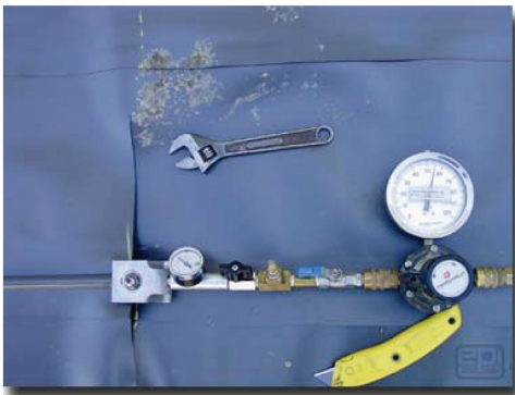
Figure 1. PVC air channel burst testing.
