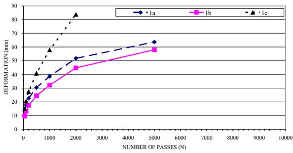
Figure 4a Trial A: Development of deformation in Lane 1
