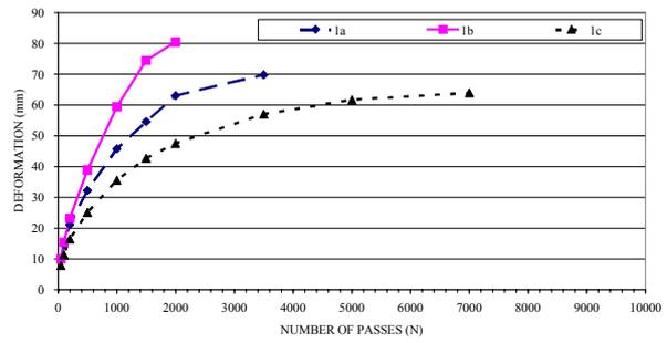
Figure 5a Trial B: Development of deformation in Lane 1
