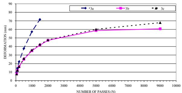
Figure 5c Trial B: Development of deformation in Lane 3
