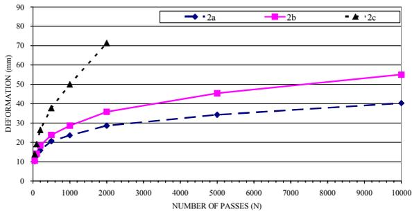
Figure 4b Trial A: Development of deformation in Lane 2
