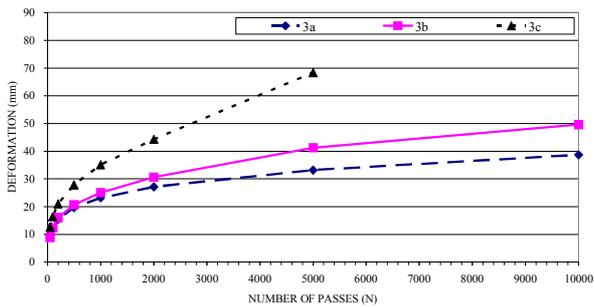
Figure 4c Trial A: Development of deformation in Lane 3
