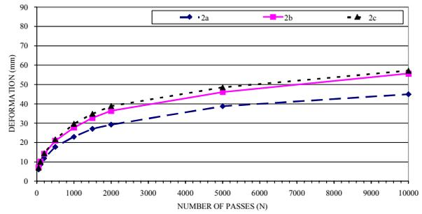
Figure 5b Trial B: Development of deformation in Lane 2
