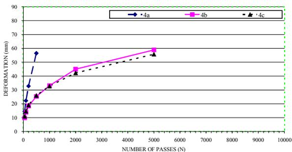
Figure 4d Trial A: Development of deformation in Lane 4
