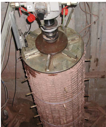
Figure 2: Geogrid reinforced stone column in one dimension compression test
