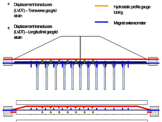
Figure 5 Schematic plan and cross-section of the instrumented embankment
