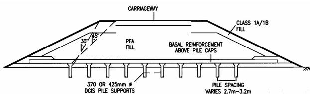
Figure 2 Pile Supported Embankment Section
