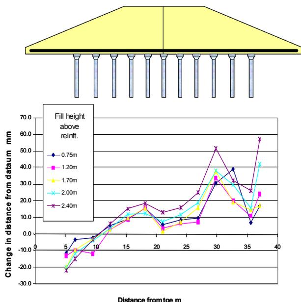
Figure 6 – Measurement of lateral spreading of the embankment
