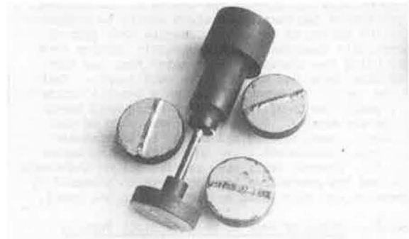
Figure (9). Modified weighted sample holder for use as Abradant.
