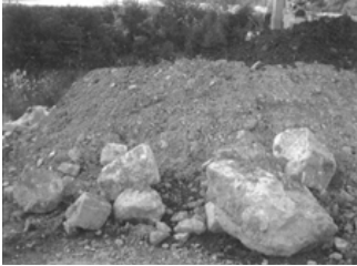
Photograph 1. Boulders in the existing fill
