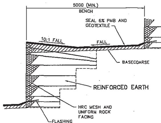
Figure 3. Details of Reinforced Earth terraces
