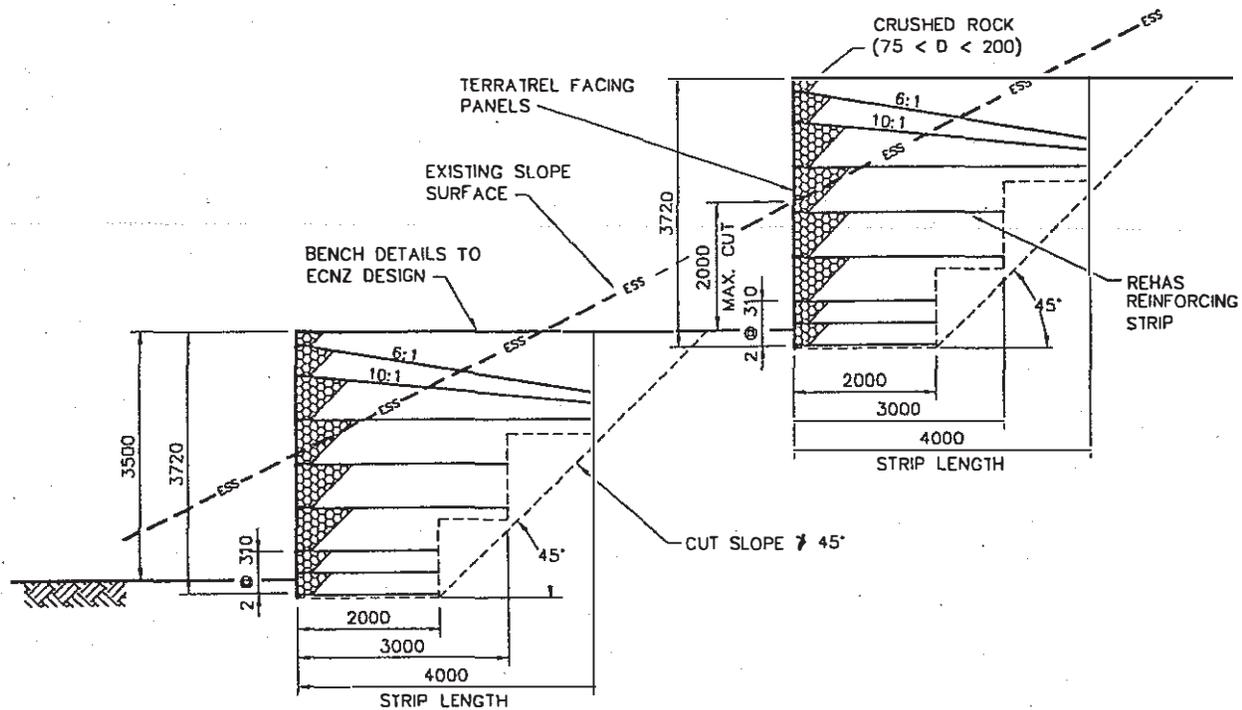
Figure 2 Cross section of Reinforced Earth terraces
