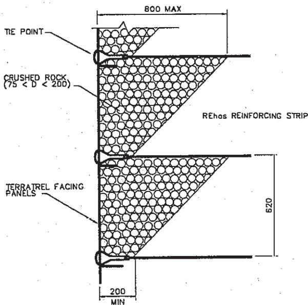
Figure 4. Details of *Terratrel* facing system
