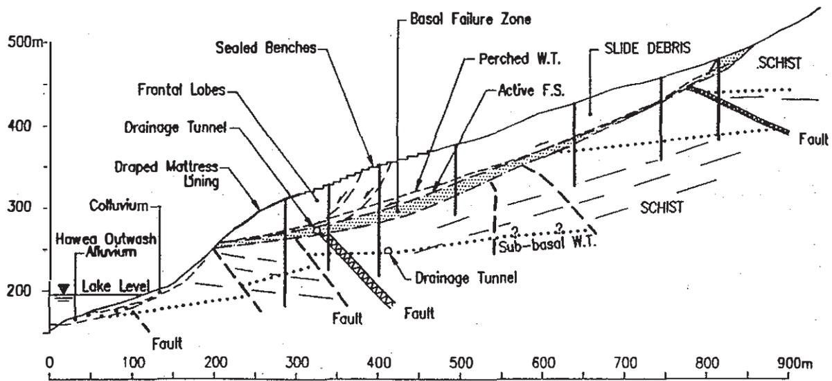
Figure 1. Cross Section of Landslide
