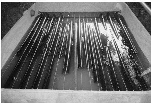
Figure 2. PVC and HDPE geomembranes immersed in the leachate
