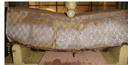
Figure 7 Beam test with geocell having opening size 50 \times 50 \times 100 mm (a) before the test and (b) after the test
