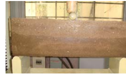
(a) Soil beam without any reinforcement (before the test)
