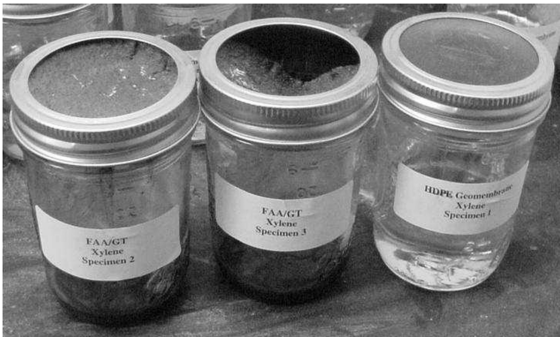
Figure 4. Solvent vapor transmission tests showing FAA-GT and HDPE geomembranes exposed to xylene.
