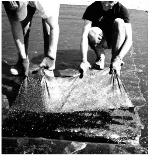
Figure 2. Sampling the field FAA-GT from the test pad.
