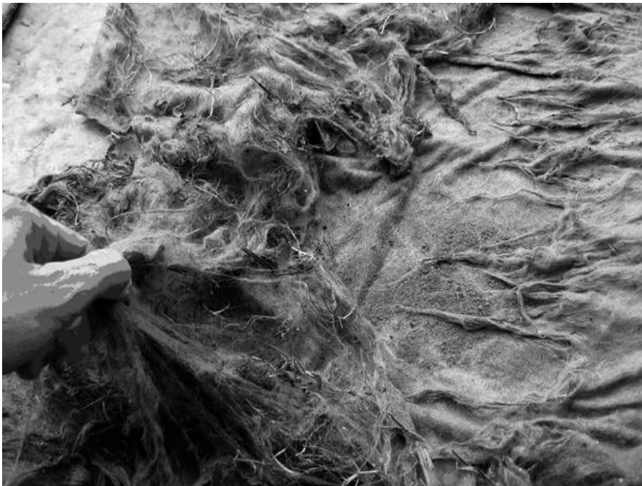
Figure 3: A geobag from the wave zone at the Bahadurabad test site at the Jamuna. The bond between the fibers is destroyed and the bag open. The bag was placed in early 1997. The photo was taken in early 2005.
