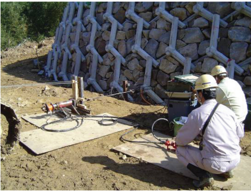
Figure 5. Setup of pull out test of block by hydraulic jacks for 4m-high test wall (Nov. 2004).
