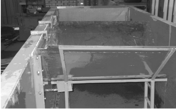
Figure 3. A side view of the canal and arrangement of drainage tank
