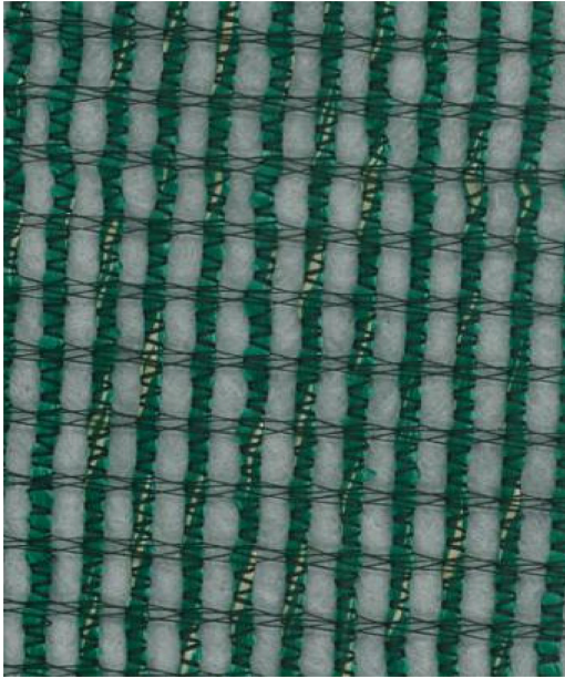
Photo 3. View of the composite reinforcement geosynthetic.
