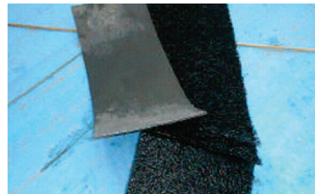
Photo 1. Geocomposite that have function of horizontal drain and airtight seat.
