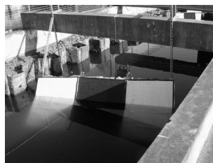
Figure 3 Exposure of geotextile samples in the tidal zone of the Circulation Basin of the Harbor and Marine Technology Research Center, Wuchi, Taichung, Taiwan
