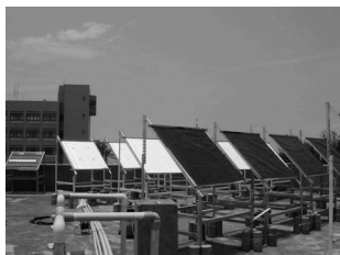
Figure 2 Exposure of geotextile samples at the top of the building of the Harbor and Marine Technology Research Center, Wuchi, Taichung, Taiwan
