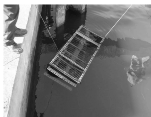
Figure 4 Immerse of geotextile samples in the Circulation Basin of the Harbor and Marine Technology Research Center, Wuchi, Taichung, Taiwan
