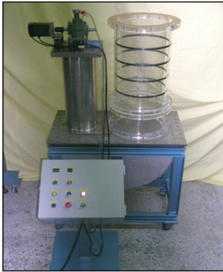
Figure 1. Front view of bi-directional cyclic flow apparatus.
