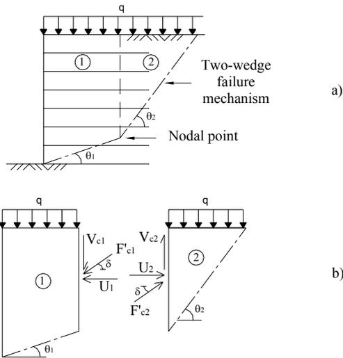
Figure 3 Two-wedge failure mechanism
