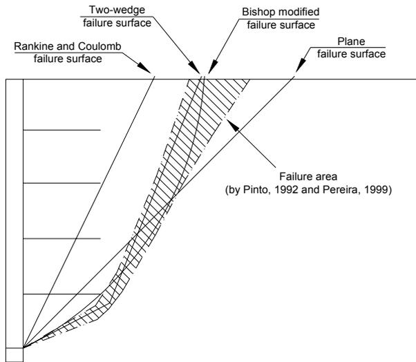
Figure 4 Failure area and critical failure surfaces predicted by different design methods for the wall 4-s
