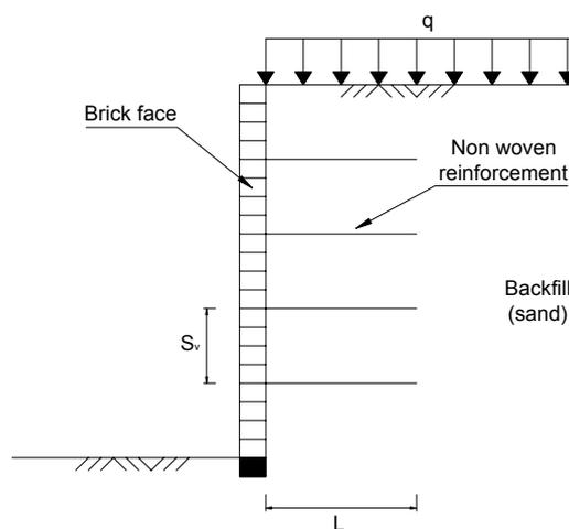
Figure 1 Brick faced reinforced retaining wall
