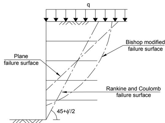
Figure 2 Failure surfaces correspondent to the different design methods used in the stability analysis
