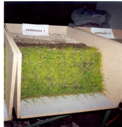
Figure 10: test arrangement 2 (burning test built into soil)
