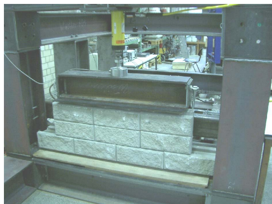
Figure 4: Photograph of the test device for SRW tests (by tBU)
