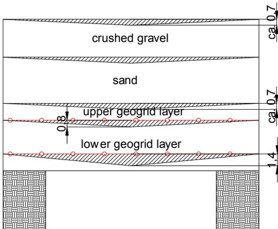
Figure 5 Depressions of the geogrid layers and of the overlying measuring planes [cm]
