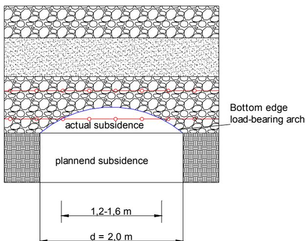
Figure 6 Actual void and assumed bottom edge of the load-bearing arch
