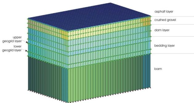
Figure 8 Model of the calculations with Sofistik®
