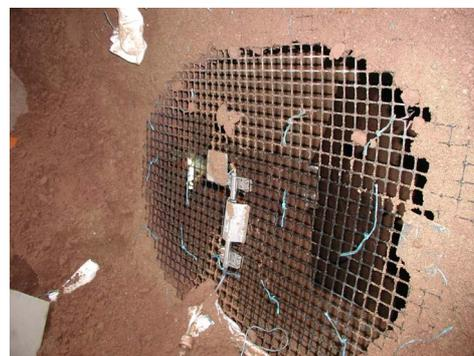
Figure 4 Exposed geogrid reinforcement after end of the test
