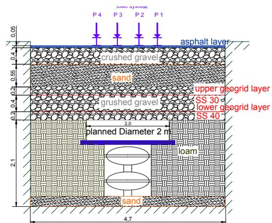
Figure 1 Longitudinal section of the trial arrangement with double-layer geogrid reinforcement.
