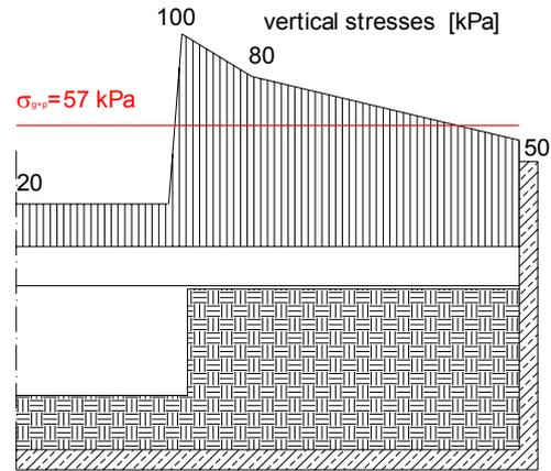
Figure 3 Vertical stresses after the end of the traffic load as planned
