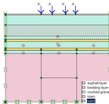
Figure 7 Model of the layers for the calculations with Plaxis®
