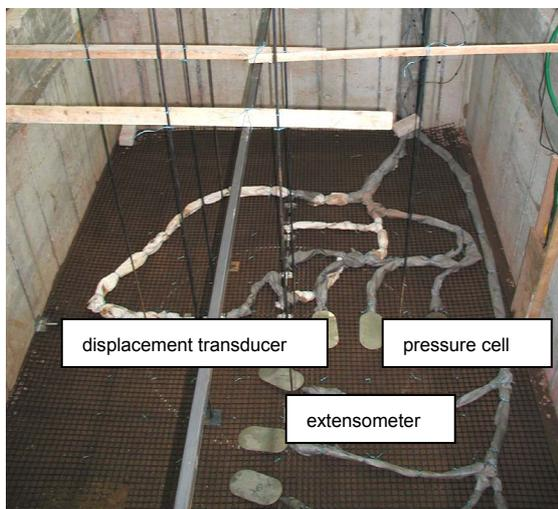
Figure 2 Geogrid and measuring instruments
