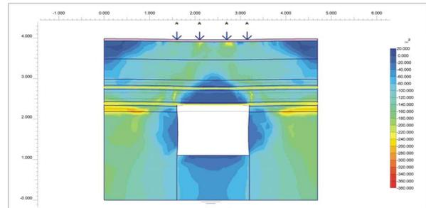
Figure 9 Calculated stress distribution using Plaxis® (additional test)
