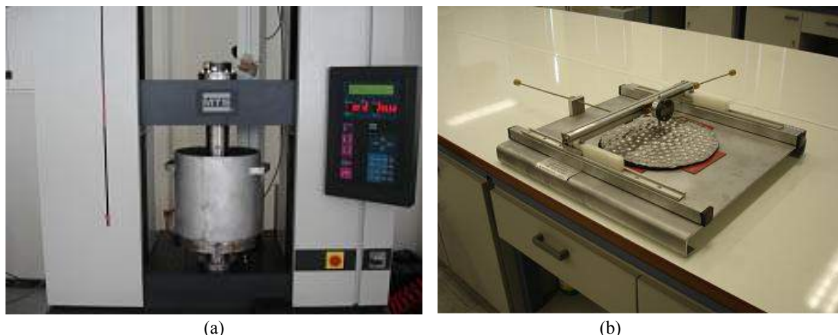
Figure 2. Long-term protection testing: (a) overall view of equipment and (b) deformation measuring system and lead plate
