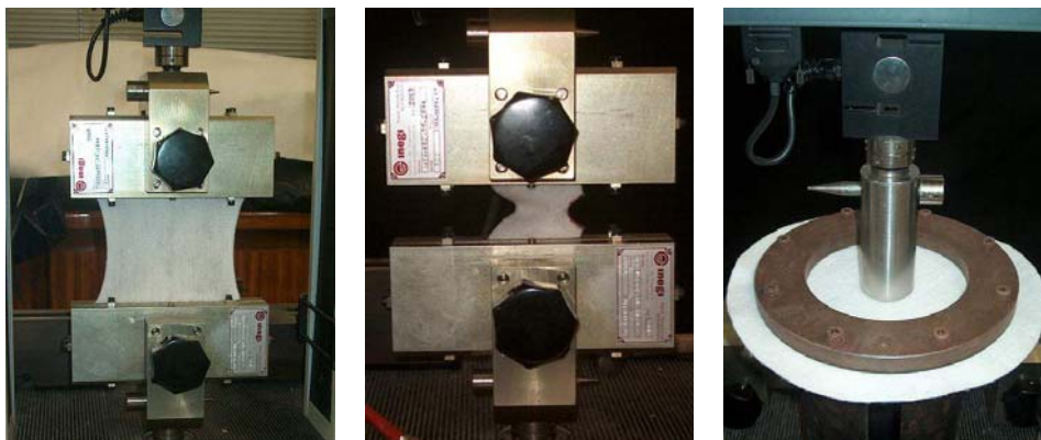
Figure 2. Mechanical characterisation of the GTXs: (a) tensile test; (b) tearing test; (c) static puncture test
