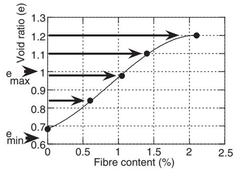
Figure 2. Maximum amount of fibres that can be mixed with a fixed amount of sand without leading to a change in specimen volume using moist tamping.
