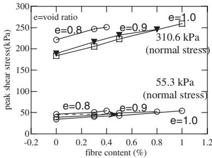
Figure 4. Evolution of the peak shear stress with fibre content, density and effective normal stress.
