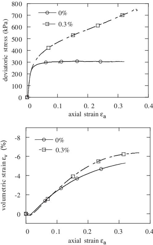
Figure 7. Stress-strain and volumetric behaviour for drained tests on D100 series specimens (legend gives the fibre content).
