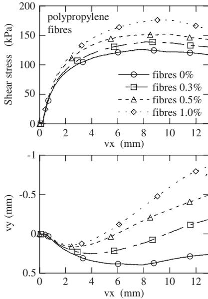
Figure 3. Typical direct shear box test results for Hostun RF sand (approximately 0% relative density) reinforced with polypropylene fibres.
