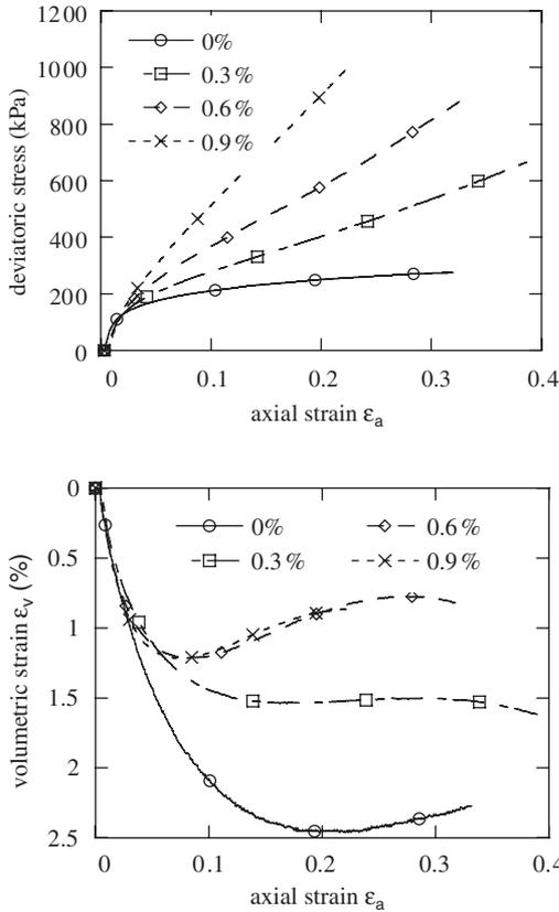
Figure 5. Stress-strain and volumetric behaviour for drained tests on L100 series specimens (legend gives the fibre content).
