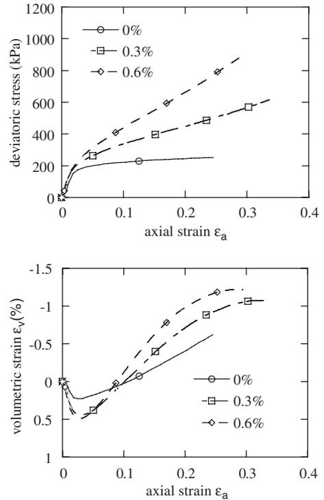
Figure 6. Stress-strain and volumetric behaviour for drained tests on M100 series specimens (legend gives the fibre content).
