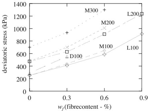
Figure 8. Trend of the deviatoric stress at 20% strain versus the fibre content for the tests performed.
