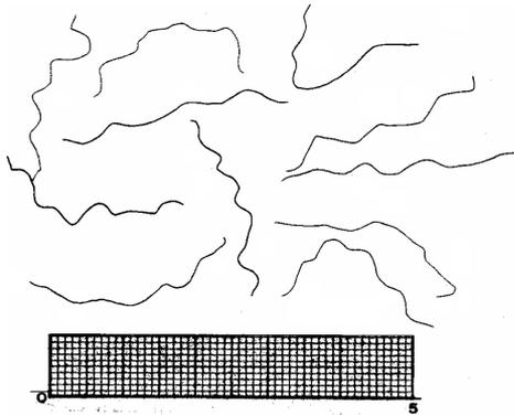
Figure 1. Specimen of individual crimped polypropylene fibres (scale in mm).
