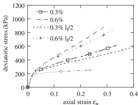
Figure 10. Influence of fibre length on the stress strain relationship on M100 specimens (legend express fibre content and fibre length).
