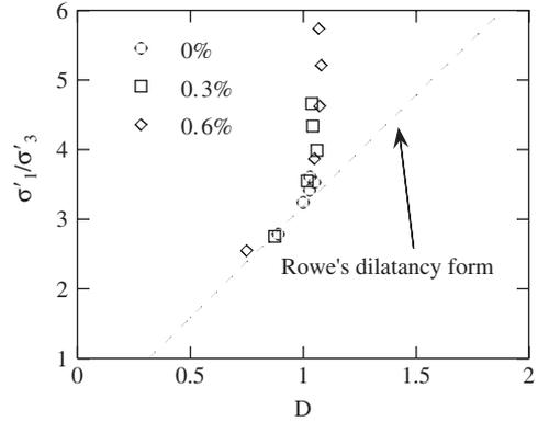
Figure 9. Stress dilatancy ratio for the test series M200 (legend express fibre content).
