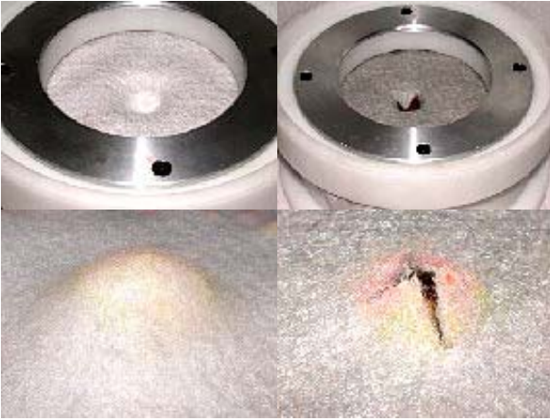
Figure 2. Results of the modified drop test with pyramid piston for two different type of geotextile.
