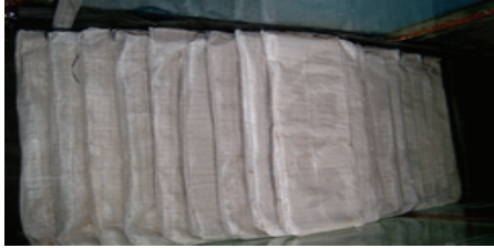
Photo.2 View of model dike piled with flat geotube
