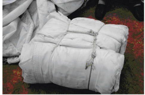
Figure 5. Larger geocontainers as brought on the site from the factory.
