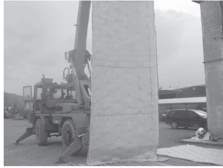
Figure 6. Lifting test on a 10 m × 2 m sample.
