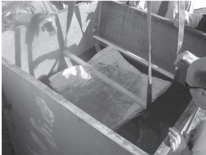
Figure 5. Determination of the BFM submerged weight.
