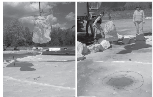
Figure 4. Impact tests on the filter mattress placed on the sandy foundation soil in dry conditions (on the left) and in submerged conditions (on the right).
